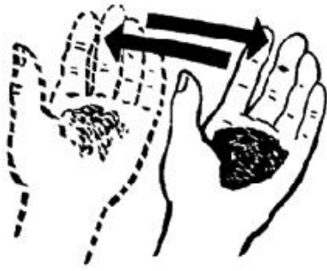
Dilatancy test: Shaking wet soil
